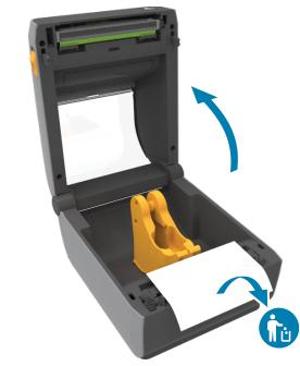
Open the printer and remove the packing.
