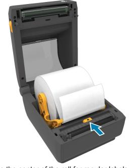
Align the sensor to the center of the roll for regular labels.
