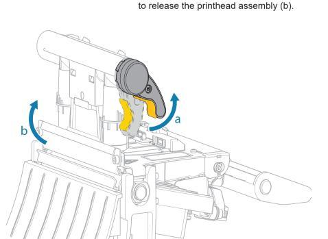
Rotate the printhead latch (a)
