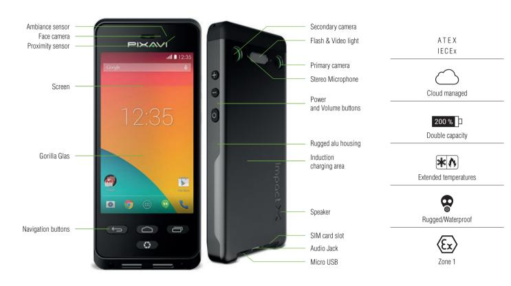
The BARTEC PIXAVI Impact X is the toughest smartphone you will ever meet. This intrinsically safe smartphone has all the functionality you will expect from a regular smartphone. The ATEX and IECEx certification has not compromised the quality and usability. The device is explosion proof and rated for use in hazardous areas. The Impact X is the next generation wireless video communication technology from BARTEC PIXAVI.
