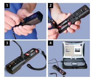
Downloading files is easy - open the rear of the camera using a coin to access the USB port. Then simply connect the camera to any PC and downloading begins automatically.
